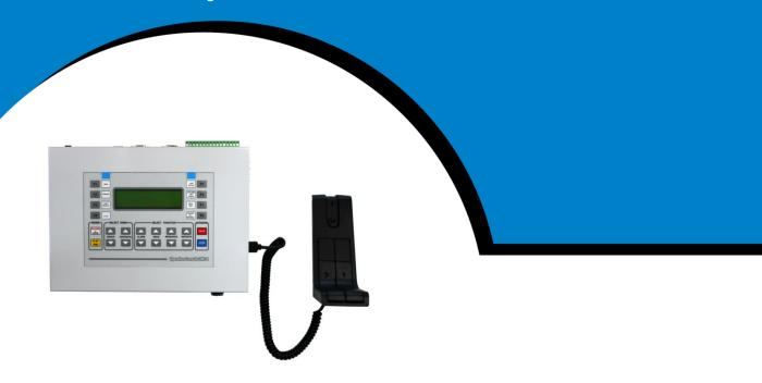
CMC 8 is a stand-alone HMI device for operating and interrogating large CS and SB series sirens and PAGA systems developed in response to users who wished to avoid a siren control system based on a PC Work Station. CMC 8 can be used as a wired remote console to control sirens for a distance up to 1000m via a dedicated Serial Data Cable (RS485). The console can also be connected to a VHF/UHF radio base station or other communication media equipment such as fibre optics networks.
