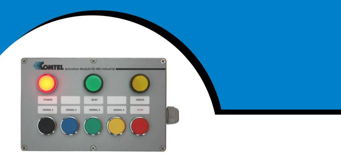
AM-10S activation panel is used to activate alarm tones/stored messages (not Live Audio) for CS and SB series sirens. It is built in a sealed enclosure and it is connected to a siren or to a siren group on a Comtel bus up to a maximum distance 1000m via a dedicated Serial Data Cable (RS485).
